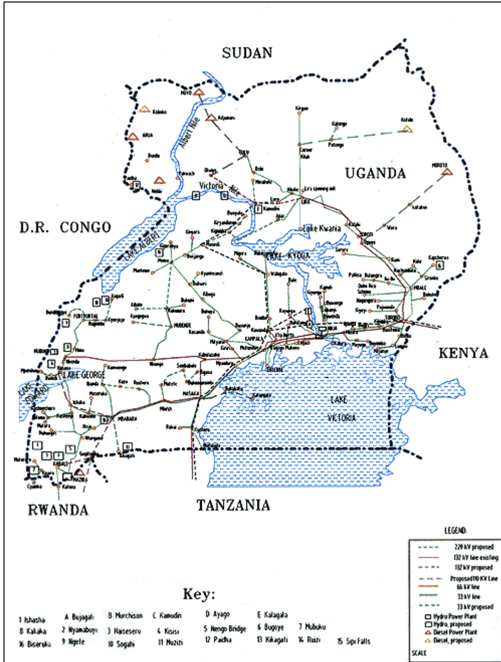
Figure 1: Uganda's Electricity Distribution Network
