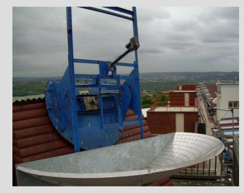
The big challenge in the construction of the concentrator is to achieve a good parabolic shape due to curvature in different regions of the parabola. For this, it is convenient to construct a dish reflecting surface by using small elementary mirrors (tiles) compared to using a single continuous mirror. Therefore, the concentrator in this research work is composed by trapezoidal tiles of an acrylic mirror material. The concentrator is a half-dish, with 2.4 meters of aperture diameter.
