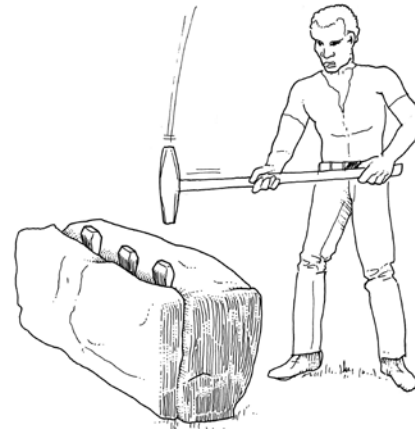
Pre-cracked rock: splitting using chis
