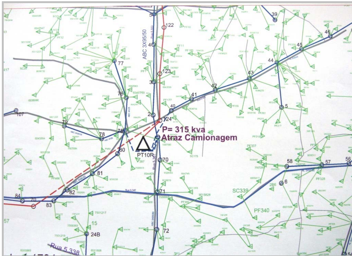
Figure 4 – Sample of Customers and Distribution Network representation by EDM GIS
