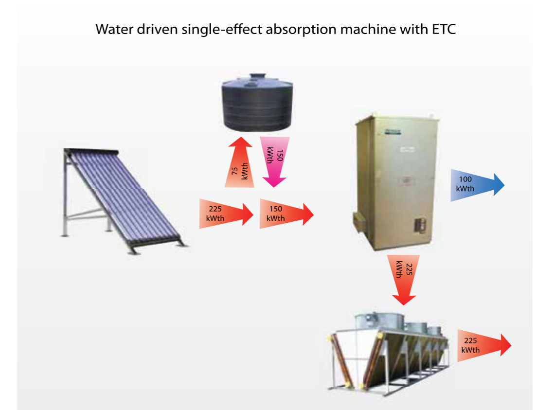
Figure 19: Sketch of an ETC-single-step system design
