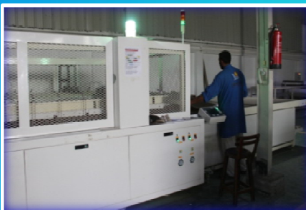
Automatic solar module laminator with capacity 16 modules per hour
