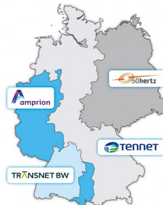
Figure 15: The four control areas and the respective Transmission System Operators in Germany (Source: SOPTIM 2015)
