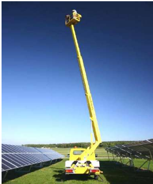
Mobile lifting platform used for infrared camera imaging
