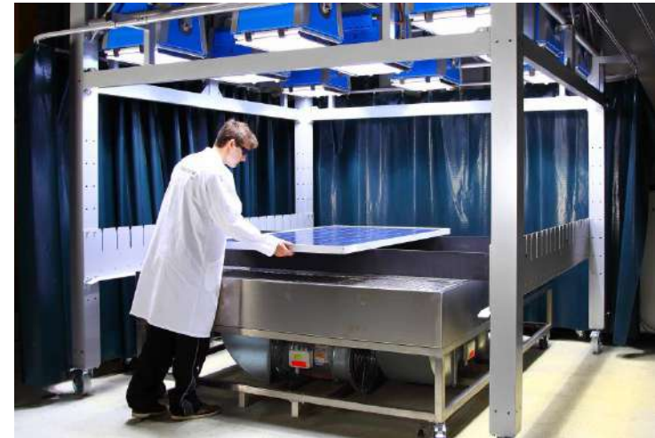
above: Continuous solar simulator for light soaking of PV modules
