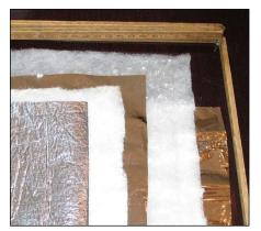
This metalized insulation foil is commonly used for pipe insulation, under laminate floors and for house insulation. It is becoming widely available.
