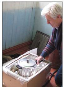
Heat-retention cookers are commonly made from insulation materials such as Expanded Polystyrene, EPS ( $\lambda$ =0.04 W/m.K), loose wool ( $\lambda$ =0.05 W/m.K), straw ( $\lambda$ =0.08 W/m.K) or even less insulating materials. However, the highly reflective metalized foils are far more effective and require less space.
