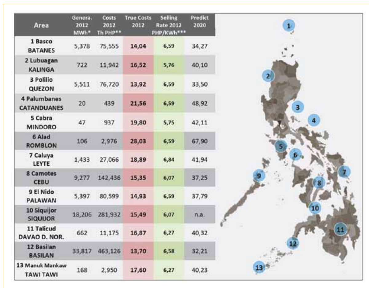
Figure 3. Overview on diesel generation, cost of generation, predictions for 2020 and electricity rates in NPC-SPUG areas * Rounded to MWh; ** rounded to Th PHP; *** rounded to two decimal figures. Source: http://www.spug.ph/MEP2012-2021.asp (May 9, 2013). Source: GIZ (2013)
