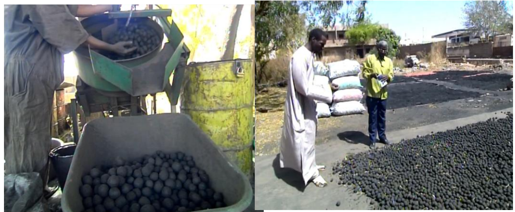
Figure 31 The agglomeration and drying process
