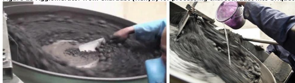
Figure 25 Agglomerator from Chardust (Kenya) for processing charcoal dust into briquettes.
