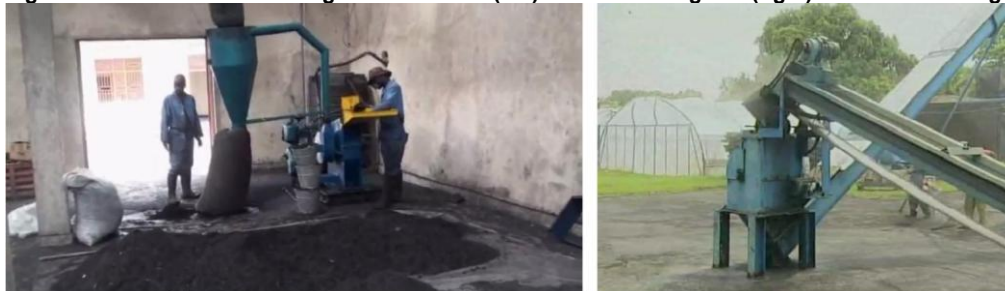
Figure 21 Hammer mill for sizing charcoal dust: (left) manual feeding and (right) automatic feeding
