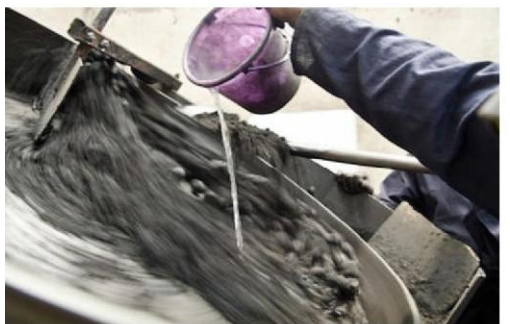
The Fireball machine turns the dust into balls by adding hot water to the mix as it turns and turns.
