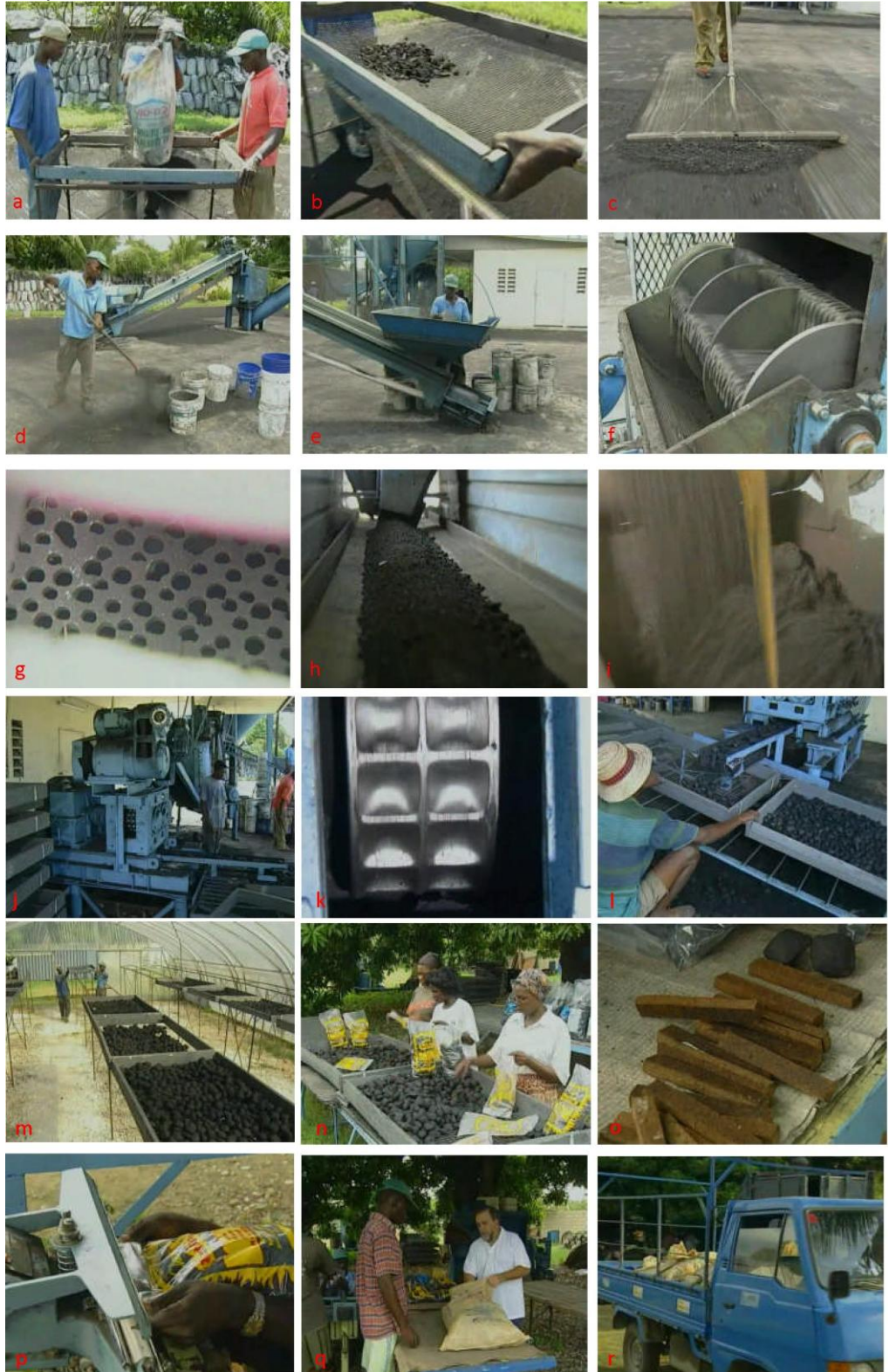
Figure 18 Charcoal dust briquetting production process in Haiti (UNEVOC 2006).
