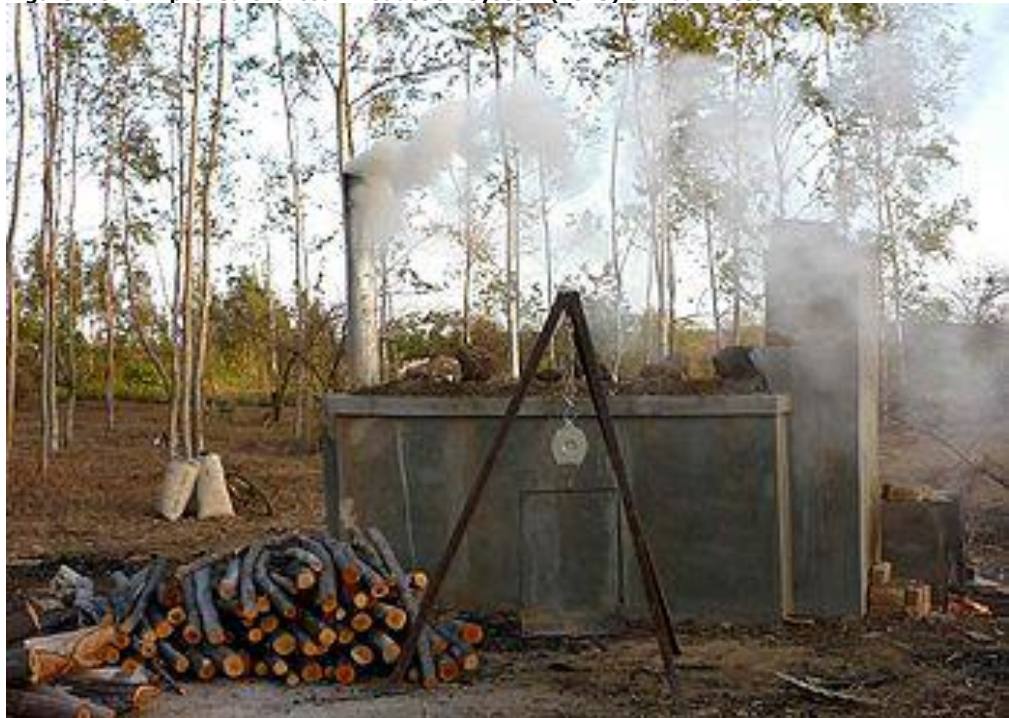
Figure 7 the Improved Charcoal Production System (ICPS) or Adam retort
