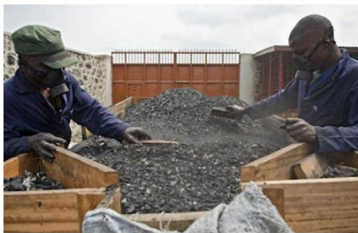
The dust is sorted to remove stones, nails, plastic and other objects that can damage the machines.
