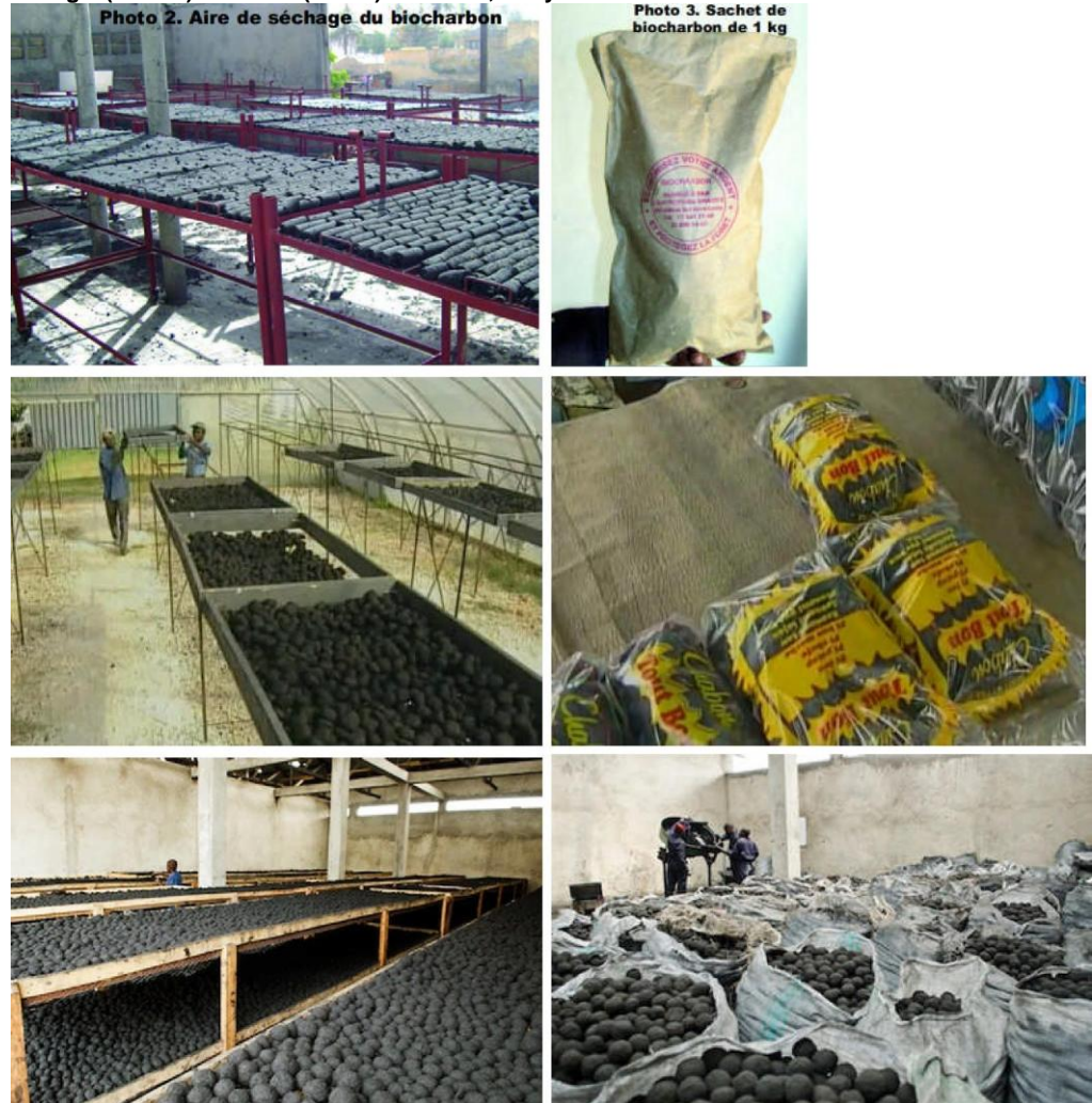
Figure 26 Drying methods for charcoal dust briquettes and bags for sale; (above) Saint-Louis, Senegal (middle) Haiti and (below) Chardust, Kenya.
