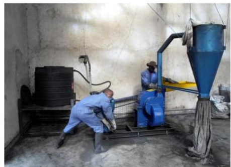
A Hammermill machine breaks the dust up into powder.
