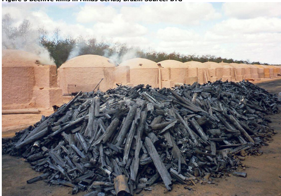
Figure 5 Beehive kilns in Minas Gerias, Brazil. Source: BTG
