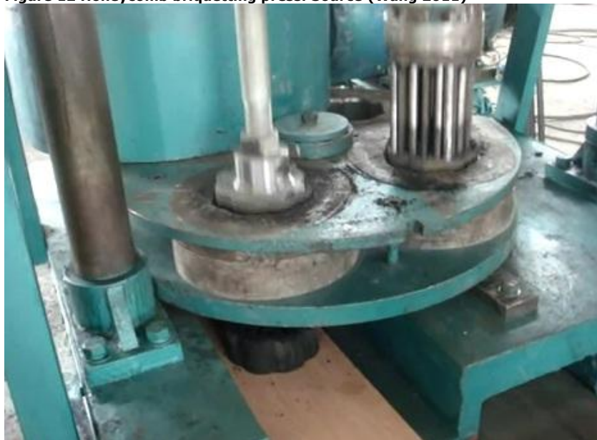
Figure 12 Honeycomb briquetting press. Source (Wang 2011)
