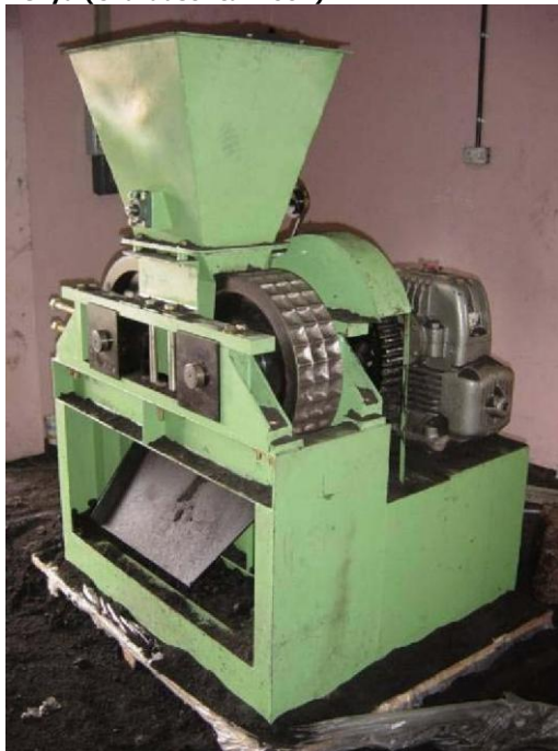
Figure 10 Roller press used by Chardust Ltd. in Kenya (Chardust Ltd. 2004)
