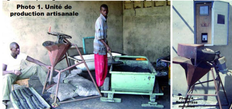
Figure 23 Briquetting charcoal dust in Saint-Louis (Senegal) using the rotor press.
