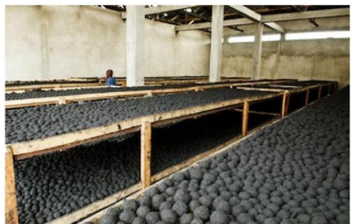
The balls are laid out on racks to dry for about 4 days, depending on the weather.
