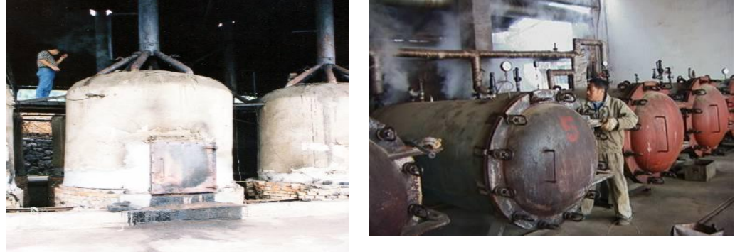
Figure 39 Bamboo carbonisation retorts in China and Japan (sources: INBAR)
