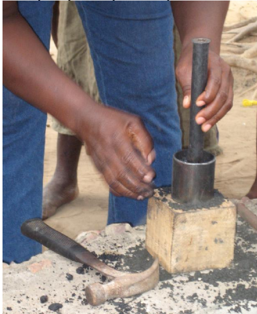
Figure 8 Charcoal briquetting using a tool developed by D-Lab (Doe 2009)
