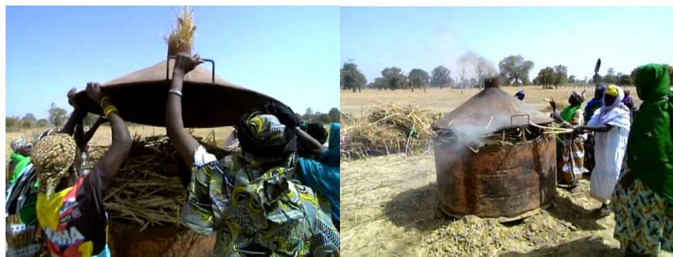
Figure 30 Closing the lid of the metal kiln, and starting the fire. Source: (Biomass Mali 2006)
