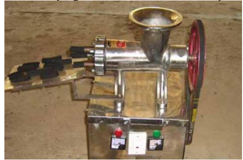
Figure 9 Meat mincer based briquetting machine (Sugumaran and Seshadri 2010)
