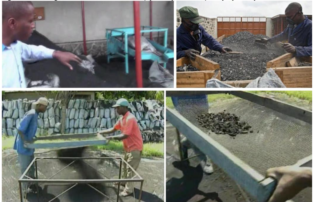
Figure 20 Sieving methods for charcoal dust; (above) Chardust, Kenya (below) Haiti.
