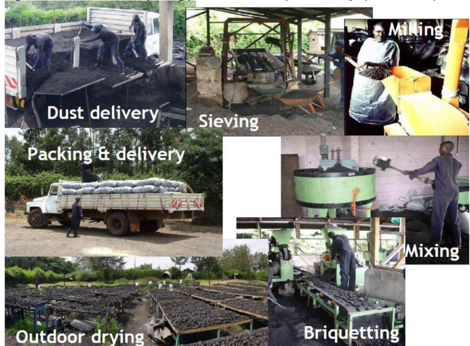
Figure 24 Charcoal dust briquetting process with roller press in Kenya (Karstad 2005)
