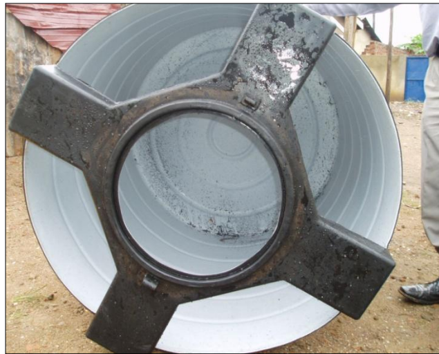
Cut the top off the GAS HOLDER tank like this
