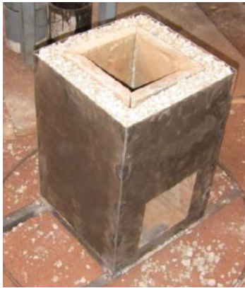
The assembled liner shown inside and outside of the metal combustion chamber box
