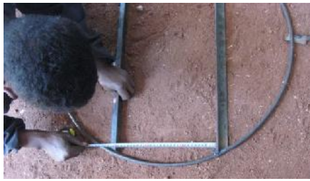
Angle iron pieces must be parallel
