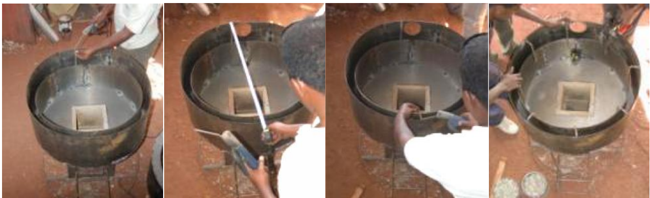
Figure 10.2 Weld the pot stabilizers to the skirt
