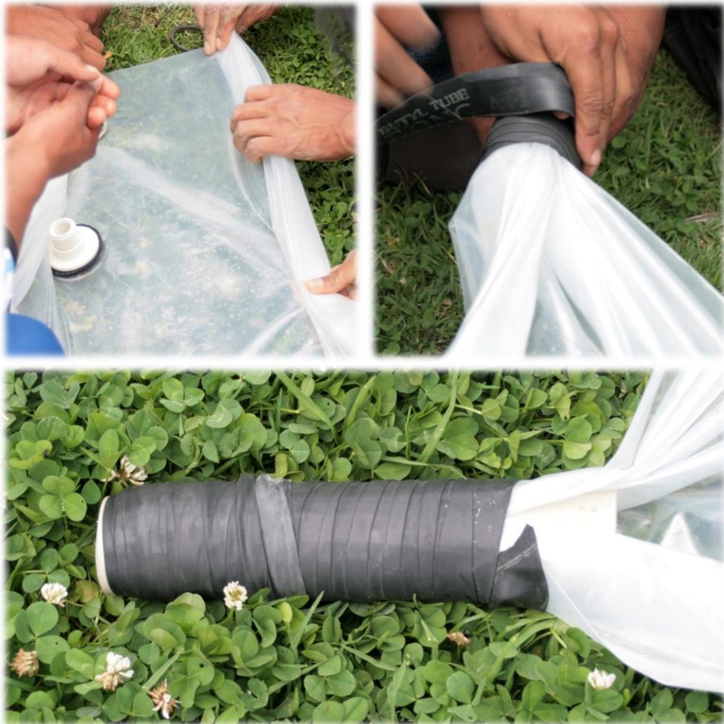
Figure 20: Bending the biogas storage reservoir with biogas outlet / flange
