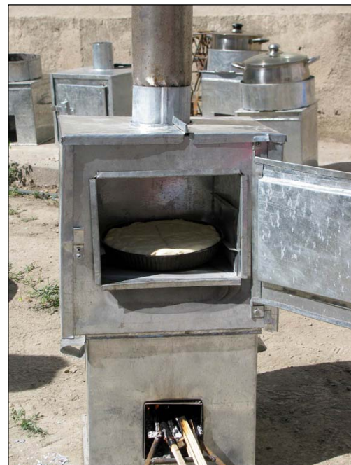
Use of the heat exchanger (left) and bread-baking oven (right, placed on an ICS, with cover). The heat exchanger works more efficiently if the oven door is open.
