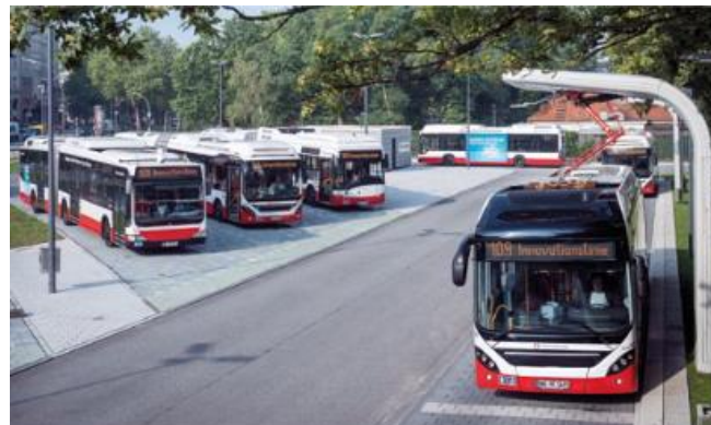
Figure 2: Opportunity charging of an urban bus at its final destination. Source: (Arbeitsgruppe Innovative Antriebe Bus)
