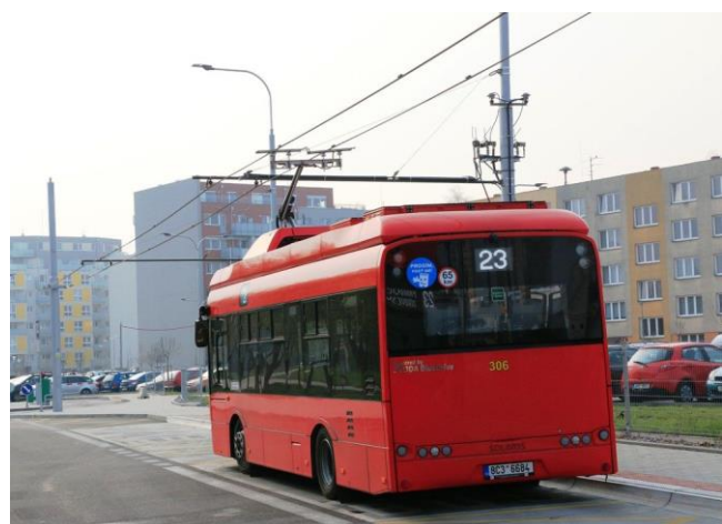
Figure 3: Opportunity charging of an urban bus using an electric road system on selected sections of the route (Source: (Harák, 2020))
