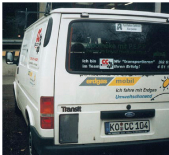
Figure 50 CNG propelled Ford Transit operating as a delivery vehicle for pharmacies in the greater Koblenz area, Germany.
