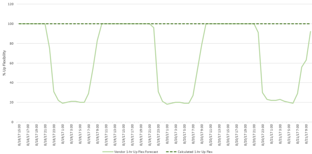
Figure 57: Vendor Forecasted and Actual Calculated Up Flexibility over 3 days for Storage Only ADER Site 2
