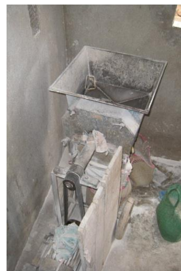
Rice mill, locally available and adaptable for charcoal milling
