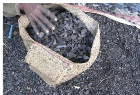
1-3 cm particles (low value) are routinely separated from sub-1 cm fines (no value)
