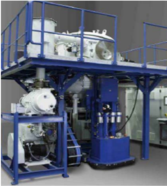
Industrial crystallization facility to produce multi-crystalline silicon ingots up to 250 kg
