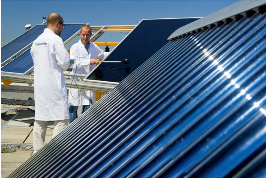
Outdoor tests as part of the complete series of tests performed on solar thermal collectors in the TestLab Solar Thermal Systems
