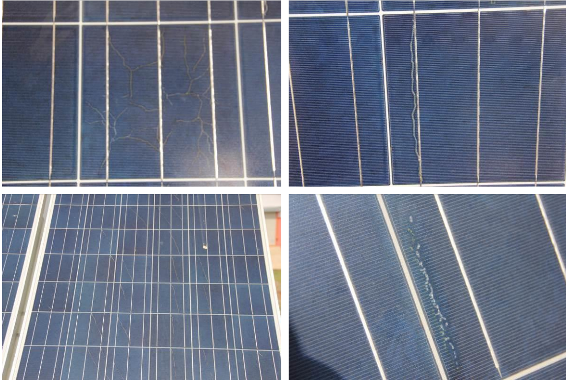
Figure 144: PV modules showing snail trails
