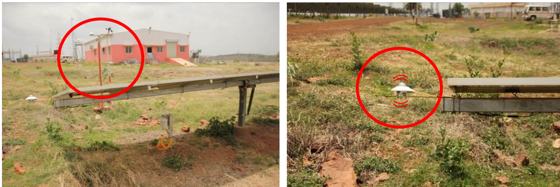
Figure 143: (left) Weather station; (right) Pyranometer
