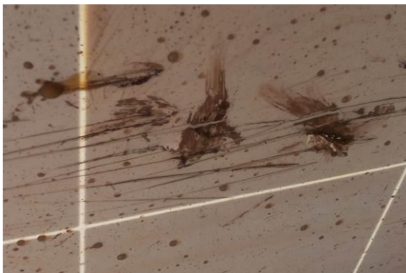
Figure 19: PV Module showing backsheet scratches [source: PI Berlin]
