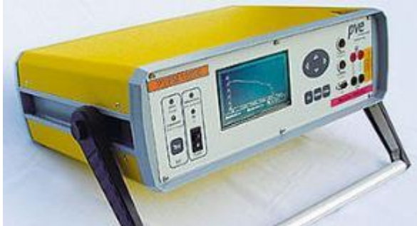
Figure 179: PVPM1000X I-V tracer [source: pv-engineering]
