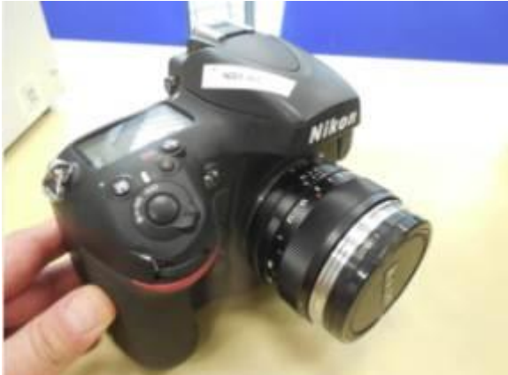
Figure 182: Nikon 800D with CCD high pass edge filter [source: PI Berlin]
