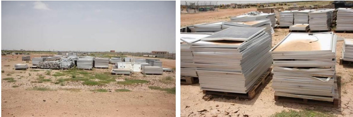
Figure 86: PV modules damaged by strong winds
