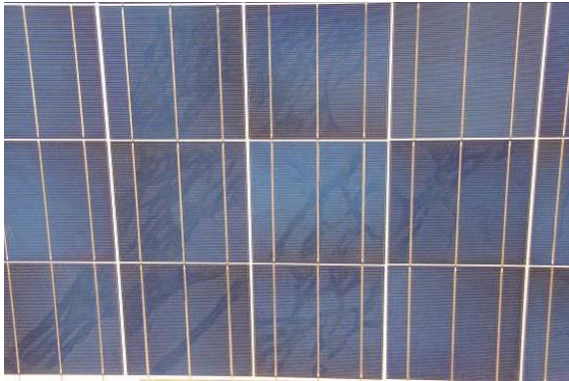
Figure 13: PV module showing snail trails [source: PI Berlin]
