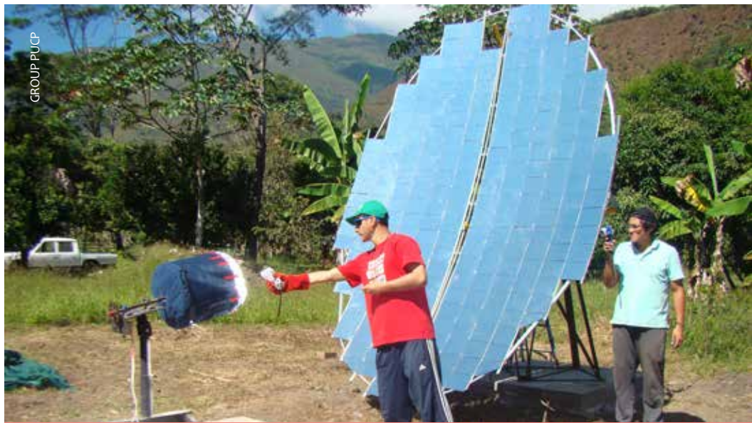
Researchers test the efficiency of a parabolic solar concentrator for cacao production.
