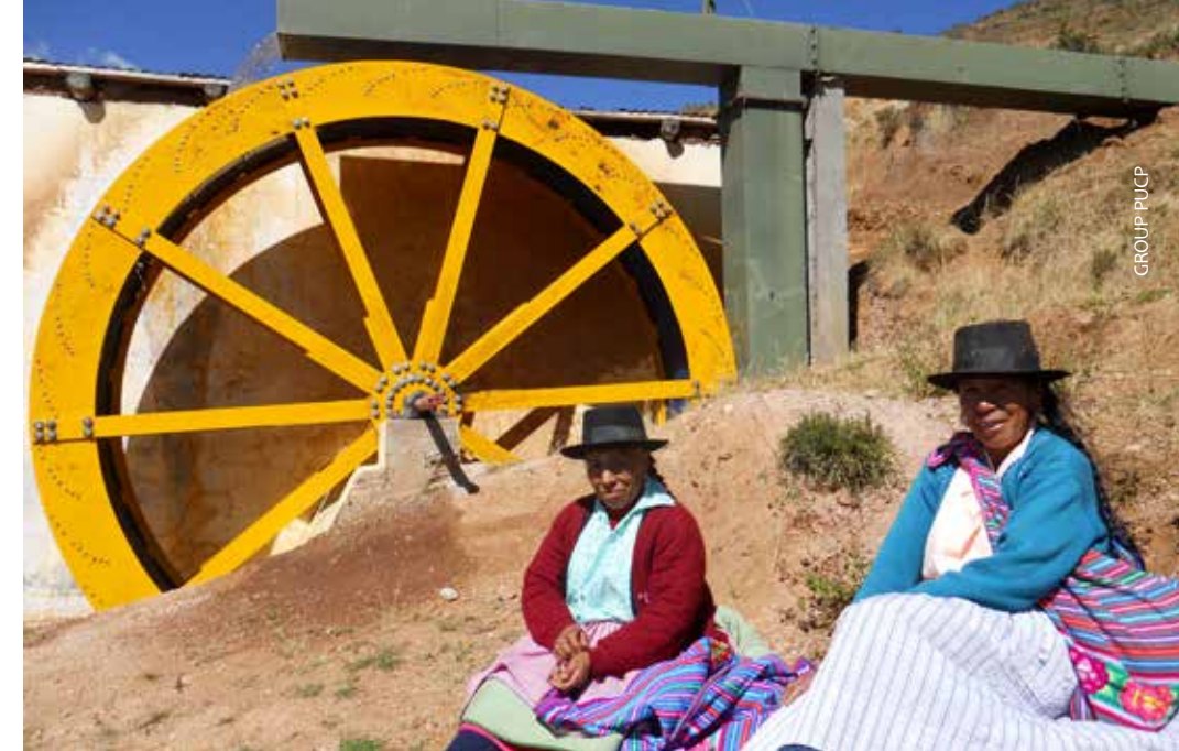
The River-generators PUCP are an alternative for electricity production in rural Andean communities.
