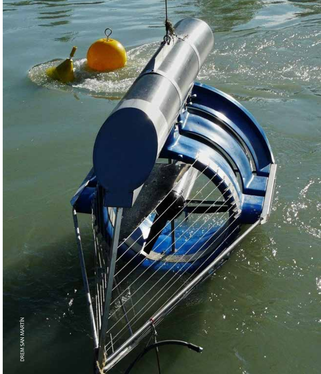
The hydro-kinetic turbine leverages the speed of current Huayabamba River in San Martin.
