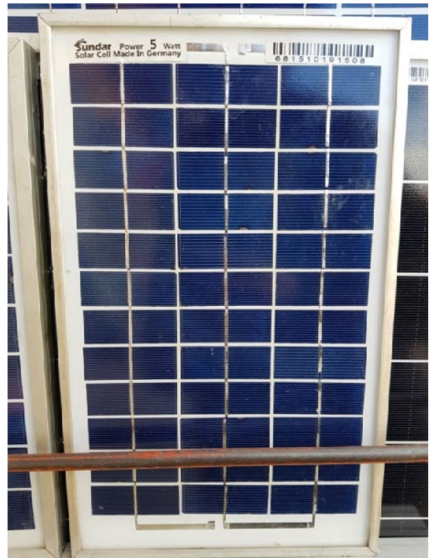
Figure 10. Low-quality PV panel with deceiving marketing (Solar Cell Made in Germany). Source: MEI
